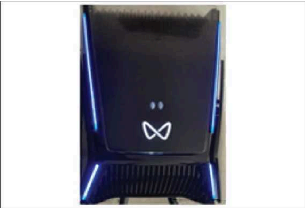
Charging in Progress , Blue color LED running pattern will glow on the charger once the charging is initiated.
