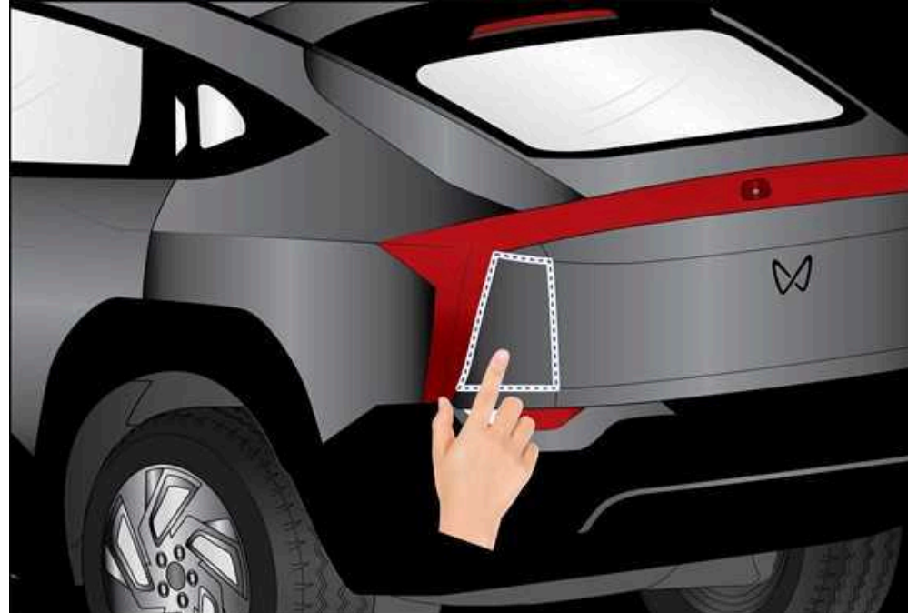
Normal Charging Port
