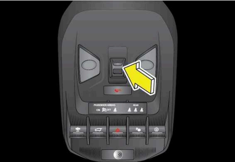
MARS Roof control switch is located on the roof console.
