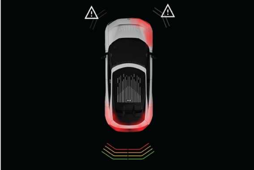
3. Obstacle in the blind zone cannot be sensed by the system. Applicable for all sensors.
